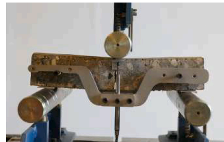
Fig. 6. Experimental set-up of the three-point bending test for determining the concrete tensile strength and mode I toughness. The notched specimen is equipped with an aluminum frame and an LVDT at the front and back sides of the specimen to measure at the point of load application the relative vertical displacement between the top and the centre of the beam.
