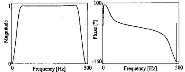
Figure 8: 8<sup>th</sup> order Yulewalk filter used for filtering accelerometer outputs
