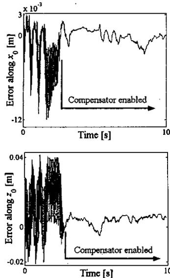
Figure 16: Cartesian errors along  $x_0$  and  $z_0$  directions
