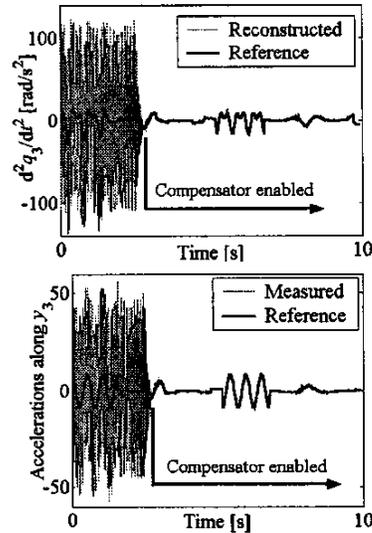
Figure 14: Left: reconstructed executed acceleration of the 3<sup>rd</sup> joint; right: measured acceleration along  $y_3$
