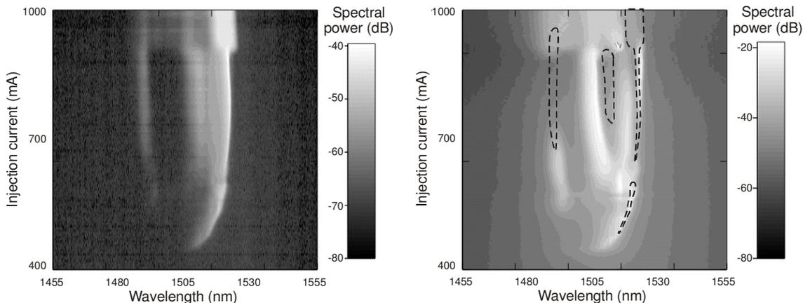
Fig. 5 Optical spectra (dB, greyscale coded) of (left) the LHS output (CCW) and (right) the RHS output (CW). The dashed line in (right) shows the position of selected maxima in (left).  $V_{SA} = -1$  V. The optical bandwidth used to obtain the spectra is 0.2 nm.
