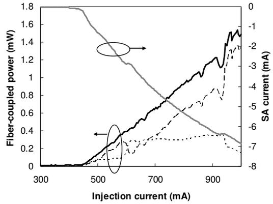
Fig. 2 Measured fiber-coupled output power for the LHS-output ( $\times 10^3$ , dashed) and RHS-output (dotted) and the calculated summation of both (solid black). The reverse bias current generated in the SA is also given (solid grey).  $V_{\text{SA}} = -1$  V.
