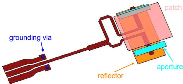
Fig. 2: A close-up view of the antenna metal structure
