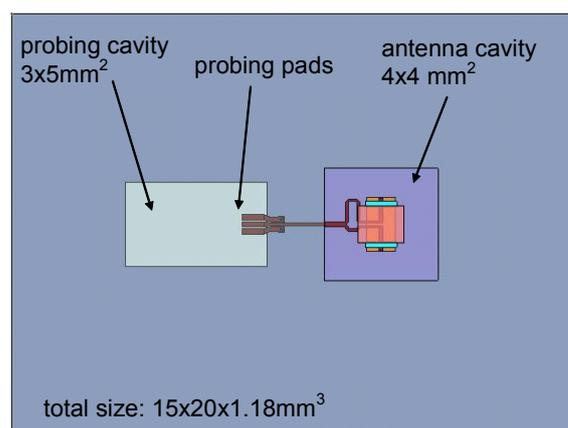
Fig. 1: A top view of the antenna structure
