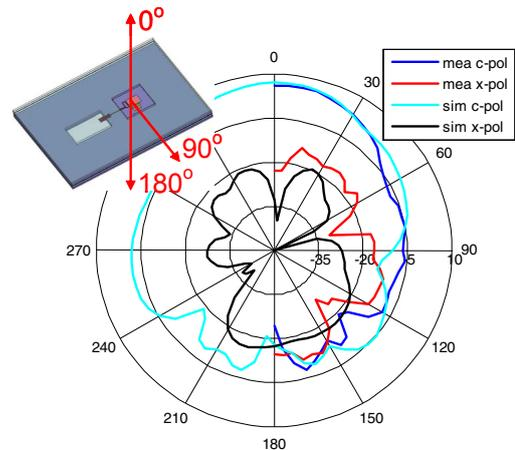
Fig. 8: Measured radiation pattern from the side (E-plane)
