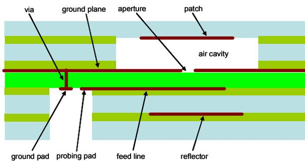
Fig. 3: Cross sectional view showing substrate layer stack-up
