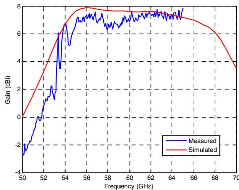
Fig. 6: Measured antenna gain
