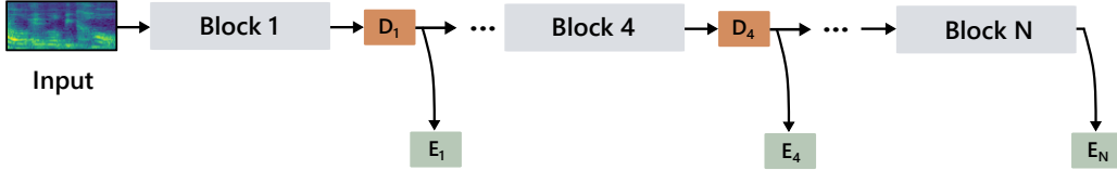
Figure 1: Overview of our early-exit binary neural networks. Grey blocks denote a set of binarized convolutional and other layers, orange and green squares denote decision exits and classification output layers, respectively. Our early-exit model enables adaptive inference for each input sample based on an entropy-based decision threshold to early-exit the input, thus saving computation.
