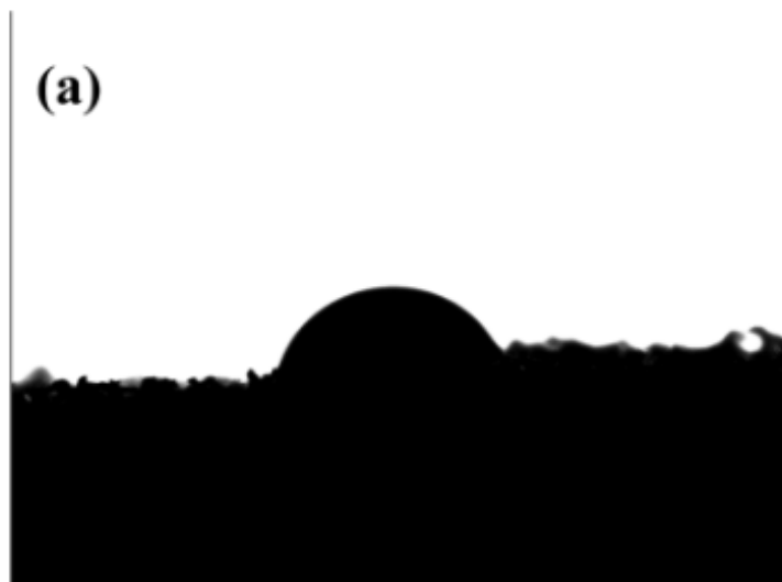
Figure 2: An image of a water droplet on a PU sponge with a contact angle of 63 degrees [16].
