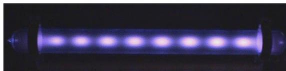
Fig. 3 A picture of the lamp at room temperature. Under these conditions stable geometric structures are easily formed.
