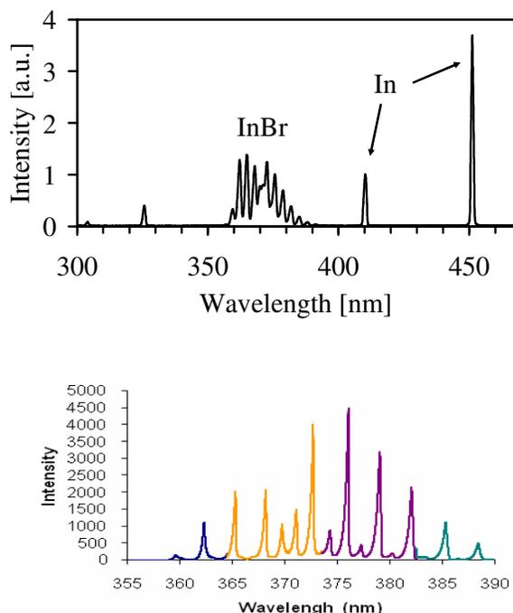
Fig. 1 Emission spectrum of InBr showing atomic lines at 410 nm and 450 nm as well as a molecular band. The lower picture shows a high resolution spectrum of the molecular band.
