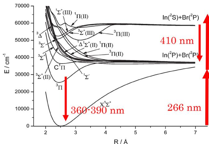
Fig. 5 Energy potential diagram of InBr (after [5]) together with the relevant laser (266 nm) and emission transitions and corresponding wavelengths (in red).
