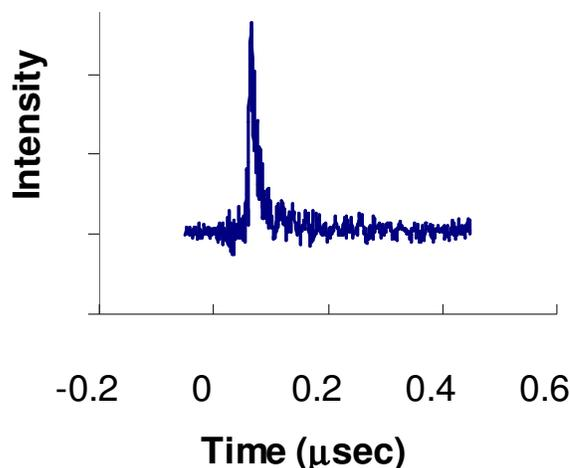
Figure 6, Laser induced fluorescence signal at 410 nm (atomic indium 2S-2P transition of fig 5). The signal is generated in a heated InBr vapor at 280°C (no plasma) in an argon buffer gas by two photon excitation using a 266 nm laser. The signal is recorded by a photomultiplier using a 1 m monochromator.
