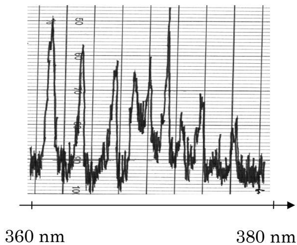
Figure 7, The 266 nm laser induced fluorescence signal of InBr observed between 360 and 380 nm (B-X and A-X transitions). The data are recorded by a photomultiplier, while scanning a 1 m monochromator. InBr is evaporated at 280°C.
