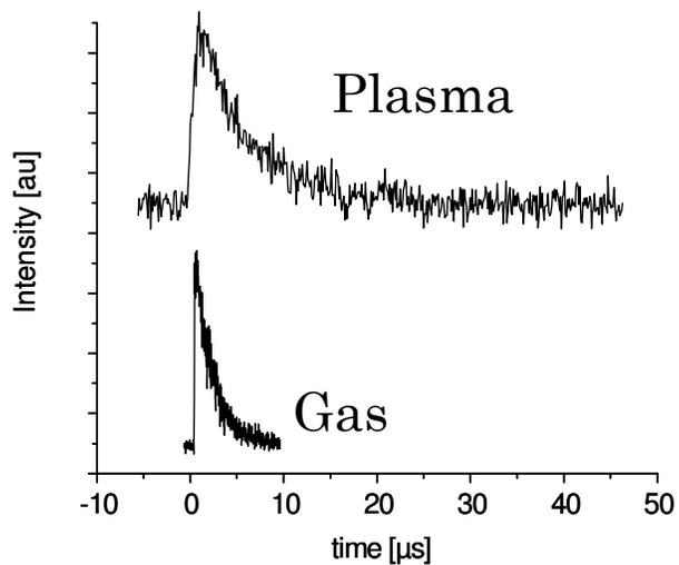
Figure 8, The time dependent 266 nm laser induced fluorescence signal of InBr observed at 364.52 nm (B-X  $\Delta v = 0$  transition). With (top) and without plasma (bottom). The amplitude of the signals is scaled and shifted.
