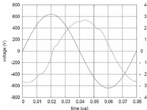
Fig. 4 Phase resolved voltage and current measurement at the electrodes of the discharge.
