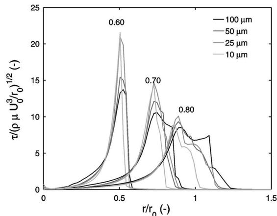
FIG. 14. Dimensionless shear stress distribution at the wall at various dimensionless times for a droplet with a velocity of 50 m/s. The four curves represent different droplet radii  $r_0$  (in microns), as indicated by the legend.
