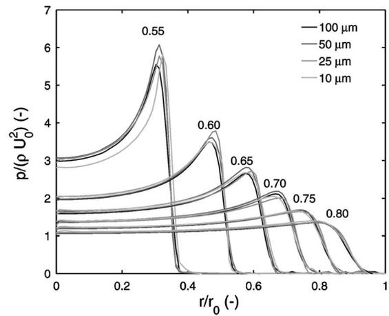
FIG. 13. Dimensionless pressure distribution at the wall at various dimensionless times for a droplet with a velocity of 50 m/s. The four curves represent different droplet radii  $r_0$  (in microns), as indicated by the legend.
