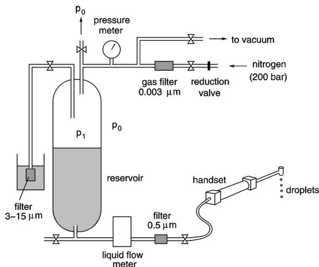
FIG. 1. Experimental setup to generate monodisperse droplets.
