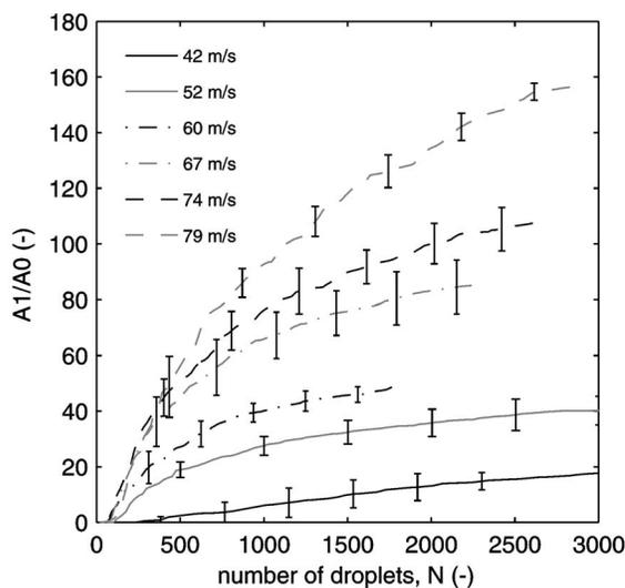
FIG. 10. Cleaned area  $A_1$  normalized with the nozzle area  $A_0$  as a function of the number of droplet impacts  $N$  for different impact velocities, indicated by the legend. Nozzle diameter equals  $50 \mu\text{m}$ . Mode of the droplet size depends on the velocity and is approximately  $100 \mu\text{m}$ ; angle of impact is  $60^\circ$ . Error bars indicate one standard deviation over 4–6 experiments.
