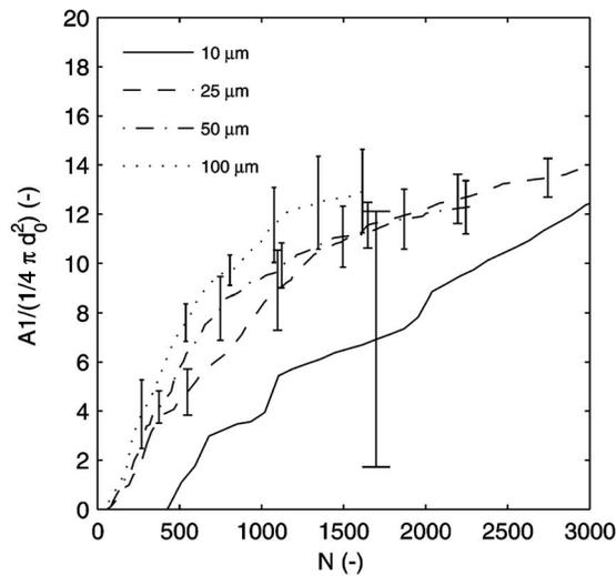
FIG. 12. Cleaned area  $A_1$  as a function of the number of droplet impacts  $N$  for different nozzle diameters, as indicated by the legend, normalized with the droplet's cross-sectional area,  $(1/4)\pi d_0^2$ . Corresponding droplet sizes are 19, 51, 92, and 163  $\mu\text{m}$ ; droplet velocity is constant,  $U_0=61\text{ m/s}$ ; angle of impact is  $60^\circ$ .
