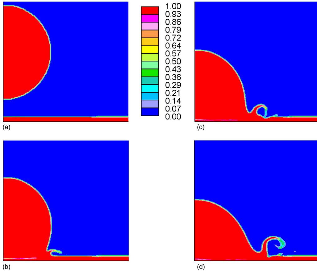
FIG. 15. (Color online) VOF fractions of an impacting water droplet with radius  $100\ \mu\text{m}$  and velocity  $50\ \text{m/s}$  on a  $10\ \mu\text{m}$  thick water film at times (a)  $t = 0.1$ , (b)  $1.5$ , (c)  $2.0$ , and (d)  $2.5\ \mu\text{s}$ .
