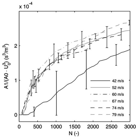
FIG. 11. Normalized cleaned area scaled with  $U_0^3$  as a function of the number of droplet impacts  $N$  for different impact velocities, indicated by the legend. Mode of the droplet size depends on the velocity, but is approximately 100  $\mu\text{m}$ ; angle of impact is  $60^\circ$ .
