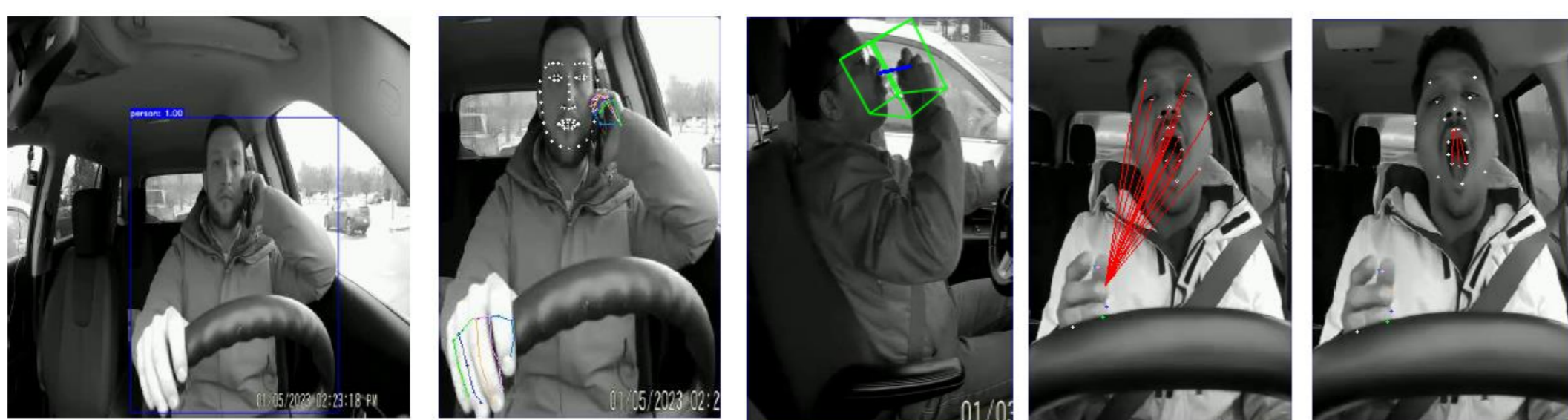
Figure 2: Top-Down pose estimation, head pose of a driver during a drinking action, relative distances between hand and face points, set of facial feature points.
