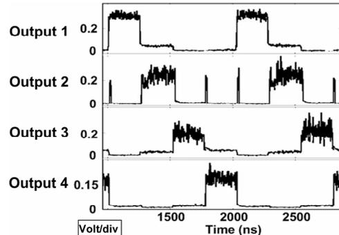
Figure 4. Switched packets at the four output ports
