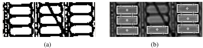
Fig. 5. Image with scratch in OLED substrate surface. Fig. 'a' shows the output after thresholding. Fig. 'b' shows the found OLEDs outlined with a rectangle. Note that OLEDs with scratch are disregarded, but should be dealt with appropriately.
