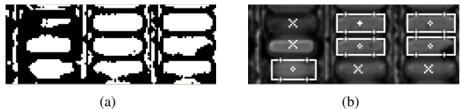
Fig. 6. Image with broken OLED structures. Fig. 'a' shows the output after thresholding. Fig. 'b' shows the found OLEDs outlined with a rectangle. The coordinates of the OLEDs that are broken are determined from surrounding OLEDs. This is necessary to ensure a continuous stream of (nine) coordinates for stable motion control. Note that some OLEDs which are broken are still found (east and south-west OLED), however, the centers are not calculated correctly.
