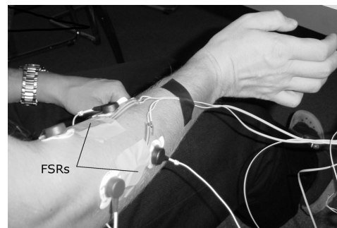
Figure 1. Placement of FSRs on the lower arm. (Larger white disks are the EMG electrodes.)
