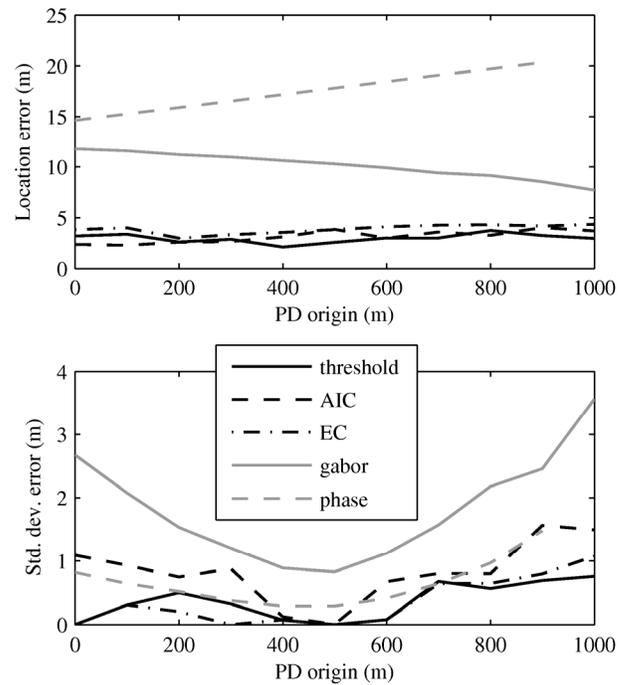
**Figure 8.** Mean and standard deviation of the location error for PDs from different locations in the cable. Load impedance at near end is an inductance of 1  $\mu$ H and the load impedance at the far end is a capacitance of 2 nF.
