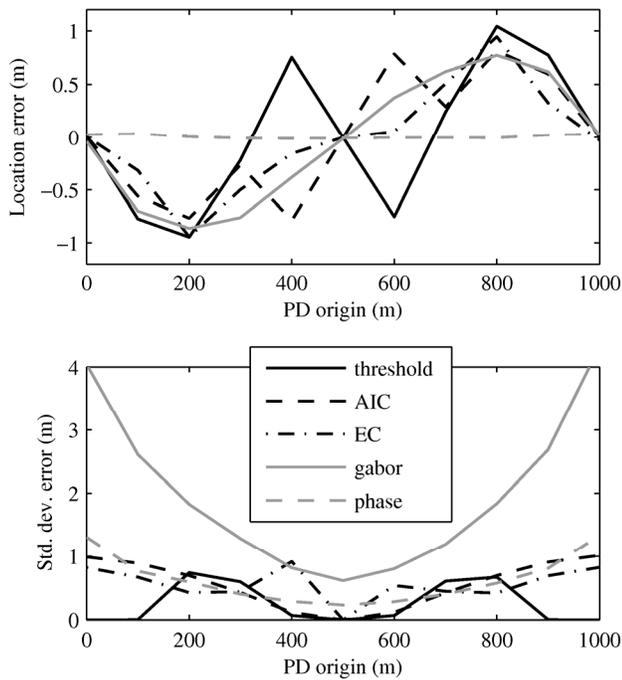
**Figure 7.** Mean and standard deviation of the location error for PDs from different locations in the cable. Load impedances at both cable ends are matched to the characteristic impedance of the cable.
