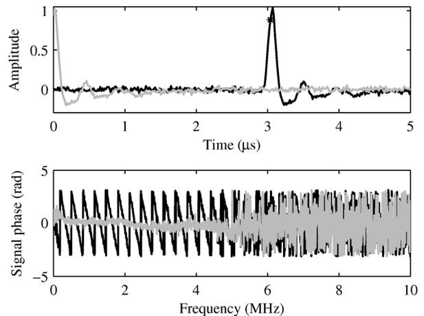
**Figure 2.** Signal before and after iteration loop. The signal is plotted in time domain and the phase in frequency domain. The iteration loop ended with  $\tau_{ch} = 3.05 \mu s$ . Black line: signal before iteration, gray line: signal after iteration loop, and \*: time-of-arrival.
