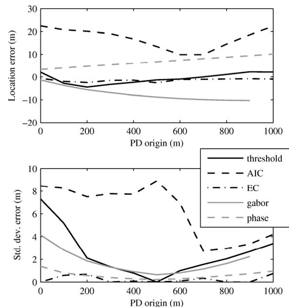
**Figure 9.** Mean and standard deviation of the location error for location of PDs from different locations in the cable. Load impedance at near end is matched to the cable and load impedance at far end is the load impedance measured in an RMU.
