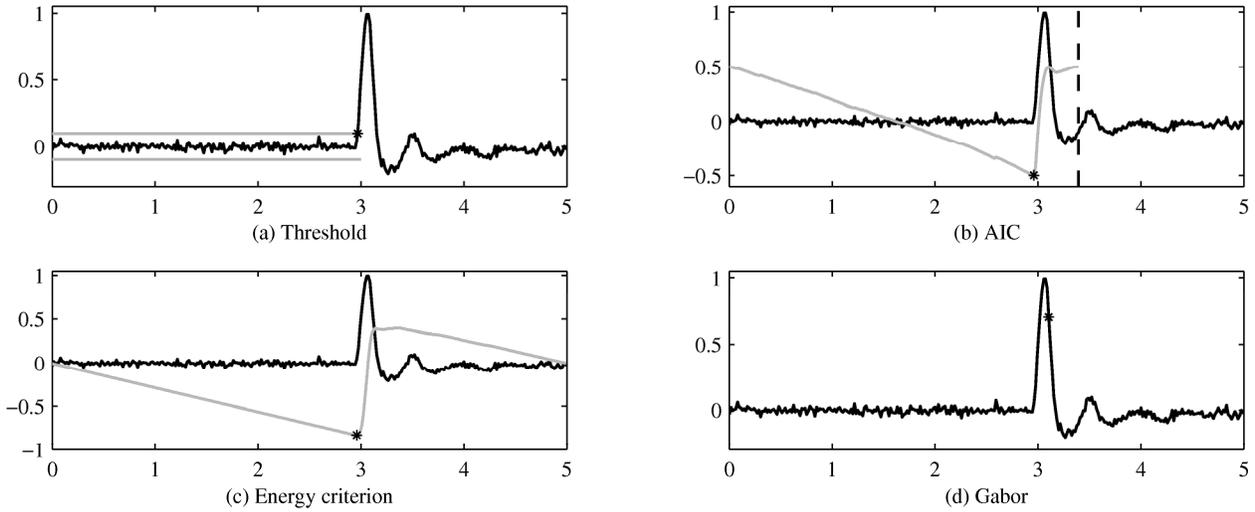
**Figure 1.** Example of recorded pulse with four  $t_{oa}$ -methods applied. Time axes are in  $\mu\text{s}$ . Black line: recorded PD signal, gray line: threshold<sup>(a)</sup> / normalized & shifted AIC curve<sup>(b)</sup> / normalized EC curve<sup>(c)</sup>, \*: time-of-arrival, and dashed line: end of record used for AIC analysis.
