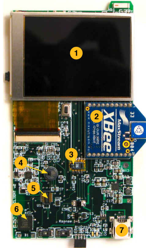
Figure 1. The Sunflower Mobile Client platform has a 320×240 pixel color display (1), humidity/temperature (3), and pressure sensors (4), and a digital compass (6). It includes a dedicated expansion connector (5), USB (7), and an 802.15.4 radio interface (2), as well as a microSD slot for flash memory or peripheral cards. The primary source of computing power is a 32-bit ARM7 implementation (AT91SAM7S256) with 64 KB of on-chip RAM and 256 KB of on-chip flash memory (on the rear side of the device), and the system is powered by a thin 2000 mAh rechargeable lithium polymer battery.
