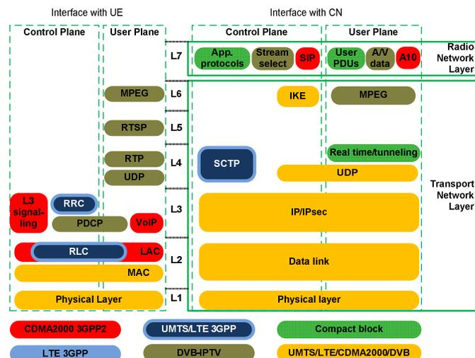
Fig. 2 DVB-IPTV extension of the HNB architecture
