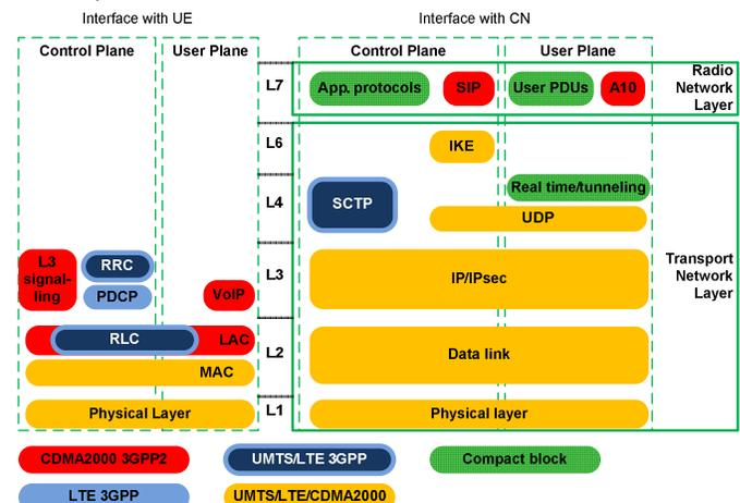
**Fig. 1 The HNB common architecture. HNB connects the user equipment (UE) with the core network (CN).**
