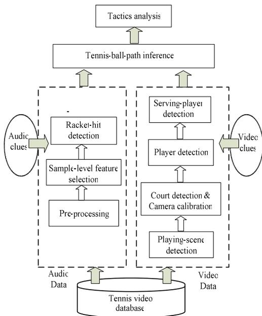
Figure 1. Block diagram of our analysis system.
