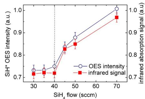
FIG. 2. (Color online) Normalized SiH\* emission intensity and SiH<sub>4</sub> infrared absorption signal at 2189 cm<sup>-1</sup> during H<sub>2</sub> plasma treatment of silicon films deposited in the large area reactor.
