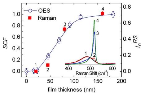
FIG. 3. (Color online) The surface crystallinity fraction SCF determined by etch product detection by OES as a function of the silicon film thickness deposited under  $\mu\text{c-Si:H}$  growth conditions on top of an  $a\text{-Si:H}$  seed layer. The data are compared to the Raman crystallinity  $I_c^{\text{RS}}$  measured at a laser wavelength of 413 nm for selected samples. The corresponding Raman spectra are shown as inset.
