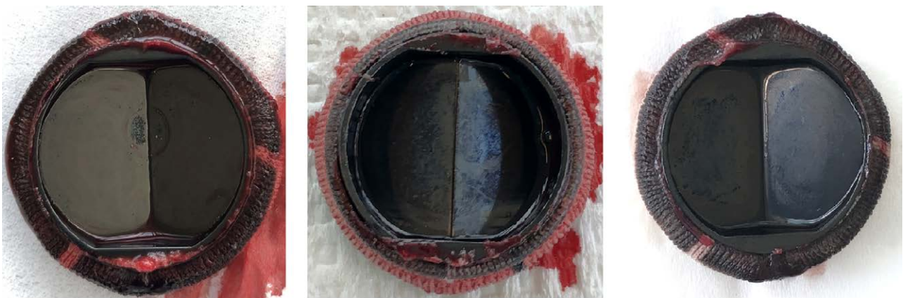
Figure 5. Thrombus formation on the mechanical heart valve after three different experiments with porcine blood in the model. Left: Test day 1, thrombus formation after the valve, mainly at 6 o'clock. Middle: Test day 2, thrombus formation before the valve, both around 12 o'clock and 6 o'clock. Right: Test day 5, thrombus formation after the valve, only at 11 o'clock.
