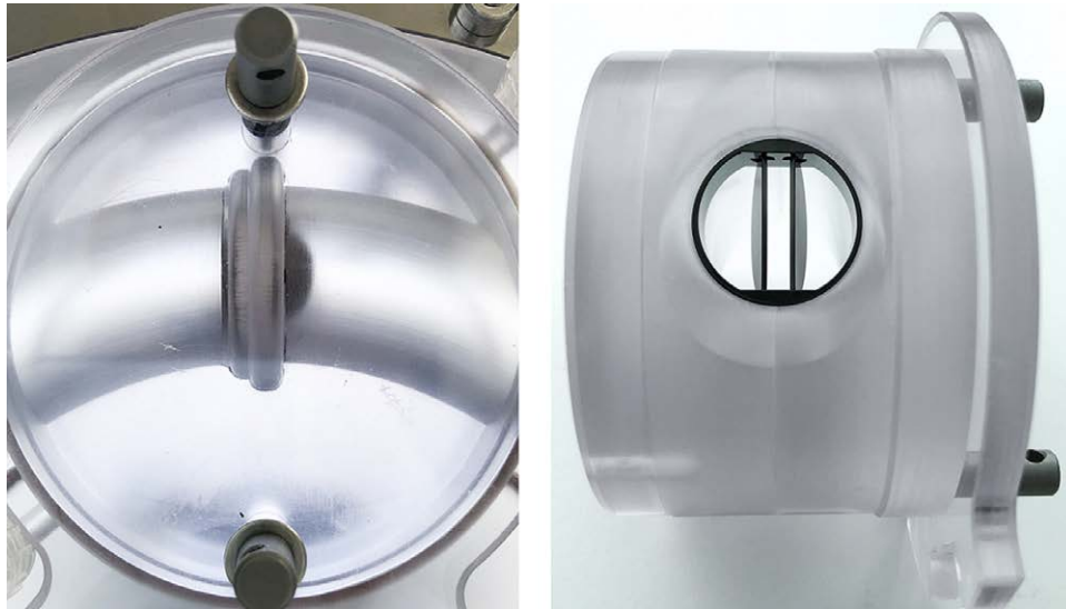
Figure 2. Valve chamber front view (left) and side view (right) showing valve positioning. Note the extra cavity for the suture ring in the left image.
