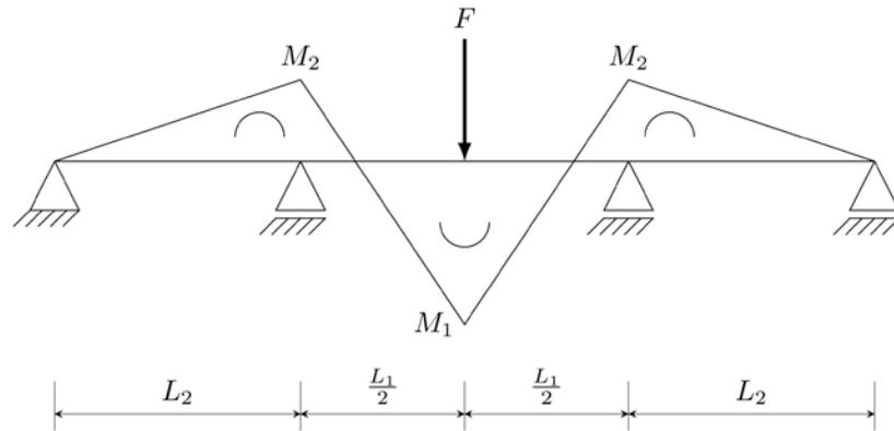
**Figure 4 The elastic moment distribution due to a single concentrated force at the centre of the middle beam.**
