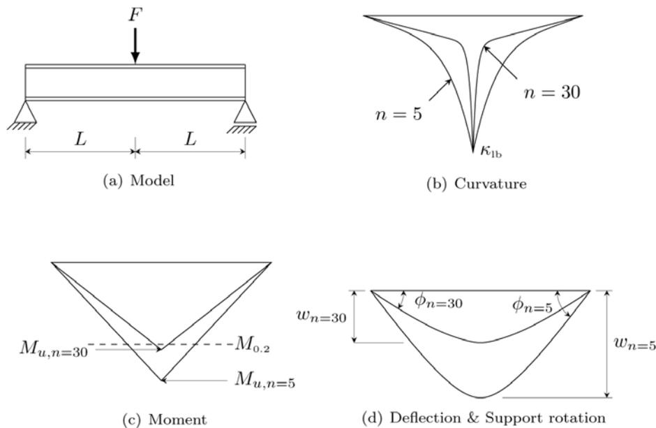
**Figure 3** The effect of curvature localisation in a simply supported beam subjected to a concentrated force at its centre.
