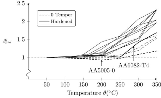
**Figure 2** The stability of aluminium alloy cross-sections at elevated temperatures. Shown here are: AA3004-H34, AA5005-0, AA5005-H14, AA6082-T4, AA6063-T5, AA5052-0, AA5052-H34, AA5083-0, AA5083-H113, AA5454-0, AA5454-H32, AA6061-T6, AA6063-T6 and AA6082-T6. After: [6].
