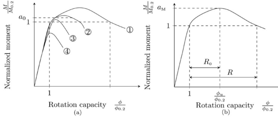
**Figure 1 (a) The 4 classes of cross-section for bending members, (b) Rotation and stable rotation capacity**
