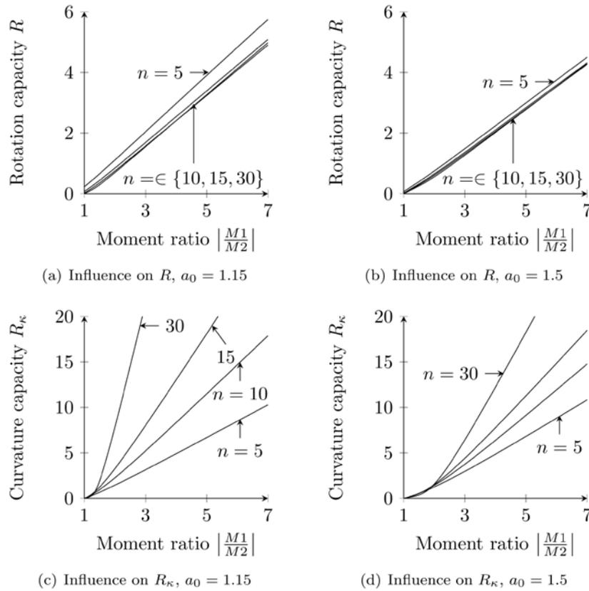
**Figure 5** The required rotation capacity (a and b) and curvature capacity (c and d) for a symmetric 3 span beam with a concentrated force at its centre with a varied middle to side span ratio expressed in terms of the ratio between the resulting elastic moments.
