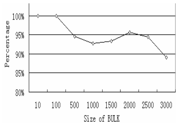
Fig. 16. Experiment 2: Percentage of received packets.
