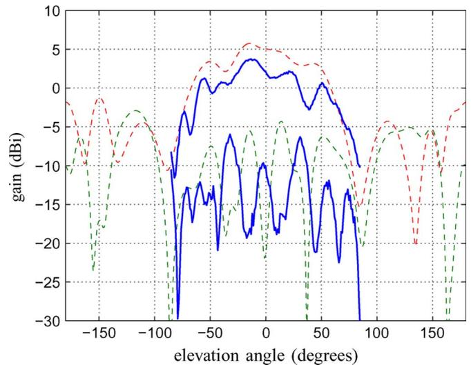
Fig. 8. Co- and cross-polarized radiation pattern of dual-polarized antenna with odd-mode excitation. Linear polarization,  $\varphi = 135^\circ$ , frequency  $f = 60$  GHz. Measurement (solid), simulation (dashed).
