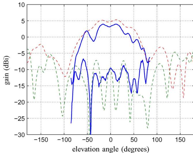
Fig. 7. Co- and cross-polarized radiation pattern of dual-polarized antenna with even-mode excitation. Linear polarization,  $\varphi = 45^\circ$ , frequency  $f = 60$  GHz. Measurement (solid), simulation (dashed).
