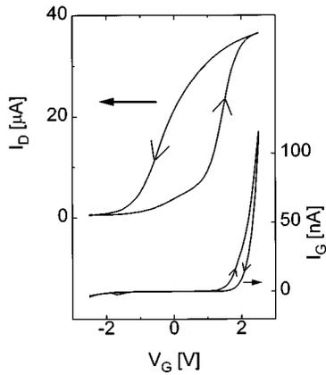
FIG. 2. Drain current ( $I_D$ ) and gate current ( $I_G$ ) vs gate voltage ( $V_G$ ). The gate voltage was swept at a rate of 2 V/s. Note the difference in the scales. The drain was at 100 mV with respect to the source. In this device, the distance between the source and drain contacts ( $L$ ) is 5  $\mu\text{m}$  and the channel width ( $W$ ) is 300  $\mu\text{m}$ .
