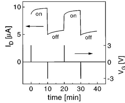
FIG. 3. Switching levels of the drain current, upon the application of gate voltage pulses with a pulse height of  $\pm 3 \text{ V}$  and a duration of 100  $\mu\text{s}$ .  $V_D = 100 \text{ mV}$ . For a device with  $L=10 \mu\text{m}$  and  $W=300 \mu\text{m}$ .
