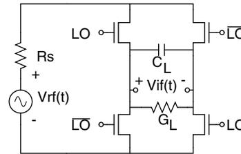
Fig. 1. Double balanced mixer circuit.
