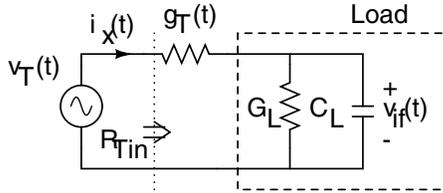
Fig. 2. Thévenin equivalent mixer circuit with load impedance.
