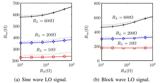
Fig. 5. Simulation and modeled input resistances.
