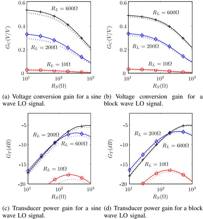
Fig. 4. Simulation and modeled voltage conversion gain and transducer power gain.
