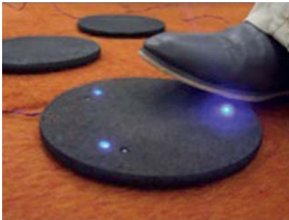
Fig. 23: FlowSteps. PhD project (TU/e), 2011. As part of the I-PE project, an initial prototype called FlowSteps is developed for an explorative study. FlowSteps consists of a large number of flexible interactive mats that players can use to throw, flip, jump or sit on. Players can create their own games by placing the mats on the floor in any position they like. The design does not communicate a clear function as the embodiment is context independent. (Credits: Rijnbout, de Valk)
