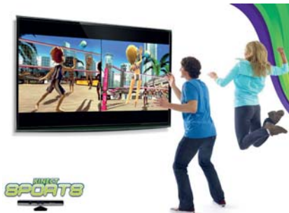
Fig. 11: Kinect for Xbox 360 . Microsoft, 2010. Microsoft Kinect for Xbox 360 is a motion sensing input device, that translates the player's physical actions into game actions. In this example the player can play volleyball, the human body as interface.
