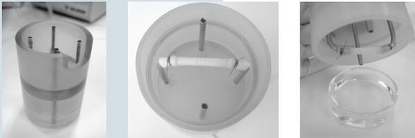
Figure 1: Bioreactor in which a shear stress and strain can be applied to tubular constructs
