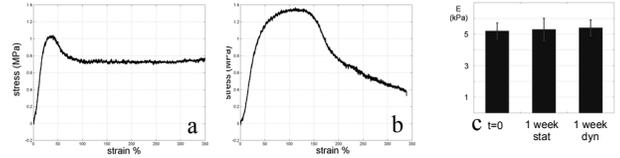
Figure 3: Stress-strain curve of PCL (a) and PCL(PEO) scaffold (b) and the resulting Young's moduli (c) under static (PBS, 37°C) and dynamic (PBS, 37°C, 7.5 % strain) culture conditions after 1 week
