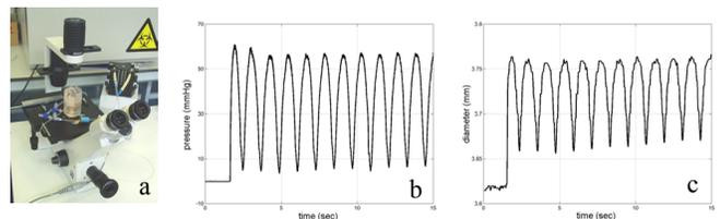
Figure 4: The bioreactor on top of a microscope (a) to measure the relationship between pressure (b) and strain(c).
