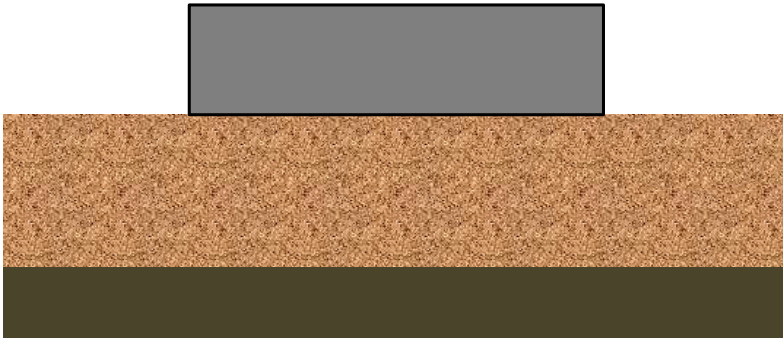
Figure 5: Schematic picture of our model of the mountain and the two soil layers. The first layer (light brown) is the soft layer. The bottom layer (dark brown) is modeled as a hard layer (not deformable), and consists of a second and third layer as mentioned below. The thickness of the layers as depicted here does not correspond to the actual ratio between them.
