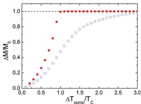
FIG. 2. (Color online) Maximum demagnetization ( $\Delta M/M_0$ ) versus laser fluence (defined in terms of  $\Delta T_{pump}$ , see text) for isolated nickel thin films of different thicknesses. Filled symbols: Optically thin film of 5 nm. Open symbols: Film of 30 nm, as used in Cheskis *et al.* (Ref. 7).
