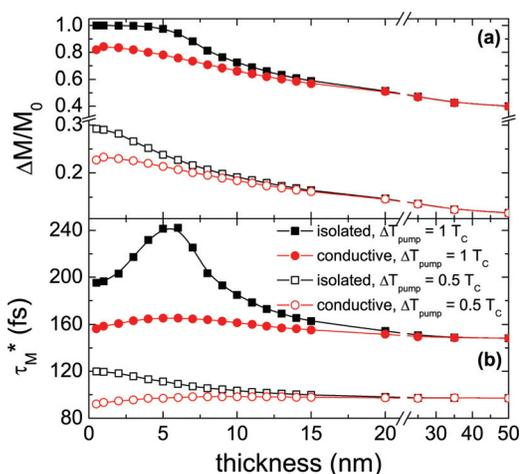
FIG. 3. (Color online) (a) Maximum demagnetization ( $\Delta M/M_0$ ) and (b) effective demagnetization time ( $\tau_M^*$ ) versus the sample thickness for two laser fluences (defined in terms of  $\Delta T_{pump}$ , see text) for isolated nickel thin film and a nonisolated nickel film (conductive structure, see text). Here, calculations were performed for an ambient temperature of 300 K.
