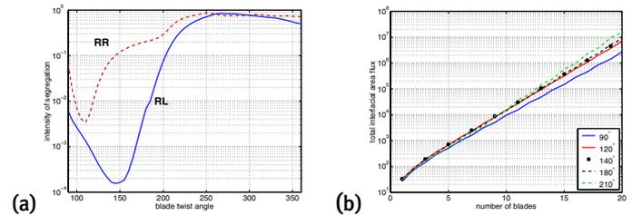
Figure 3 a) Efficiency of RL and RR Kenics mixers: intensity of segregation achieved at the cost of the pressure drop, equivalent to 12 blades of “standard” RL-180 mixer. b) The growth of the total interfacial flux with the number of blades.
