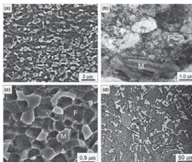
Figure 1: Microstructures of DP steels (From K.-T. Park et al., Scripta Materialia 51 (2004), 909-913).
