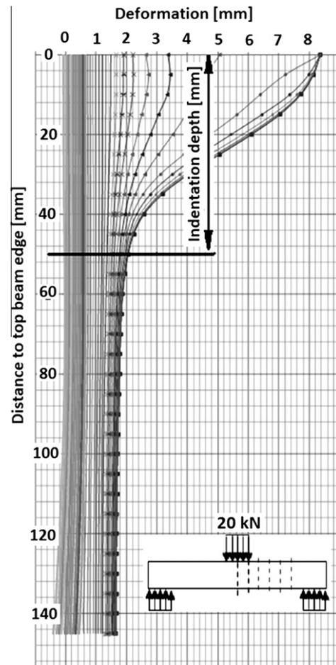
**Fig. 6.** Penetration depth of bearing stresses in consecutive cross-sections for Series A2-5.
