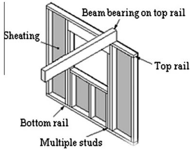
Fig. 1. Load transfer perp to grain.
