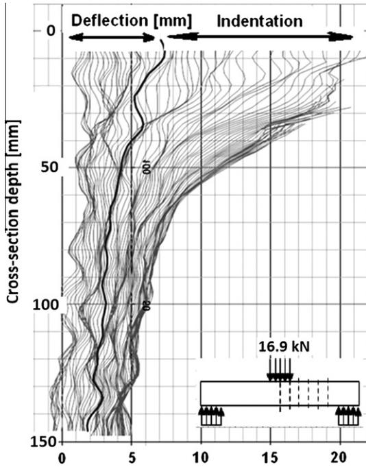
Fig. 7. Results optical detection of indentation depth.
