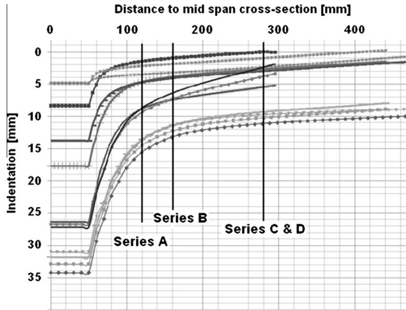
Fig. 11. FEM indentation length all test Series.
