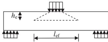
Fig. 13. Effective bearing stresses area.
