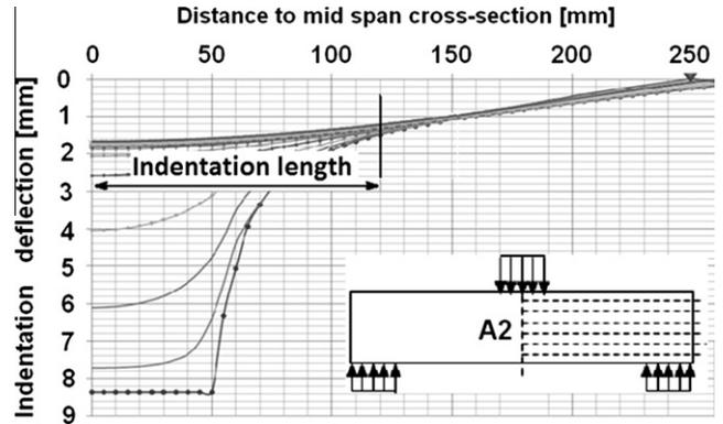
Fig. 9. Indentation length of test A2.
