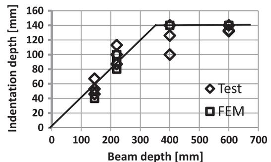
Fig. 12. Comparison FEM and optical results.
