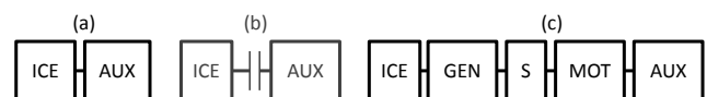
Figure 3: Topology concepts for auxiliary systems (ICE = Internal combustion engine; AUX = Auxiliary unit; S = Storage device; GEN = Generator; MOT = Motor)
