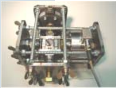
Figure 2 Prototype of high resolution discrete die with a working volume of 10x20x30 mm that consists of more than 500 discrete elements.
