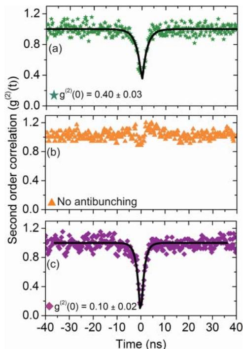
**Figure 4** | Single photon emission by a single QD in a cavity. Normalized histogram of a second-order correlation measurement  $g^{(2)}(\tau)$  after background subtraction for (a)  $XX$  (green star), (b) cavity (orange triangle) at  $T = 4$  K, and (c)  $XX$  at zero detuning,  $T = 22$  K (purple diamond). The colored symbols correspond to the filter range in Fig. 2.
