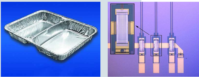
Figure 1 Two potential applications of microforming at two technological extremes: an aluminum foil container (left), and a micro-electronic device (right).
