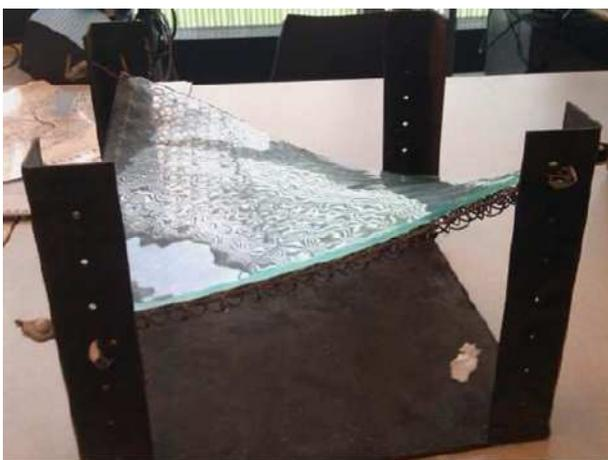
*Figure 5: Double curved glass shell on “Sierra papa 2” stainless steel mesh*
