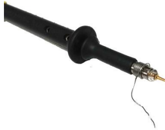
Figure 2. 5: The voltage probe to measure the ring accurately
