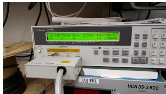
Figure 5. 1: The LCR meter testing the parameters of the inductor L_1
