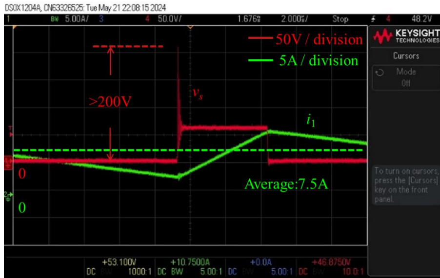
Figure 5. 5: The key waveforms of the RDC converter. (The scale for v_s is 50V per division, while the scale for i_1 is 5A.)
