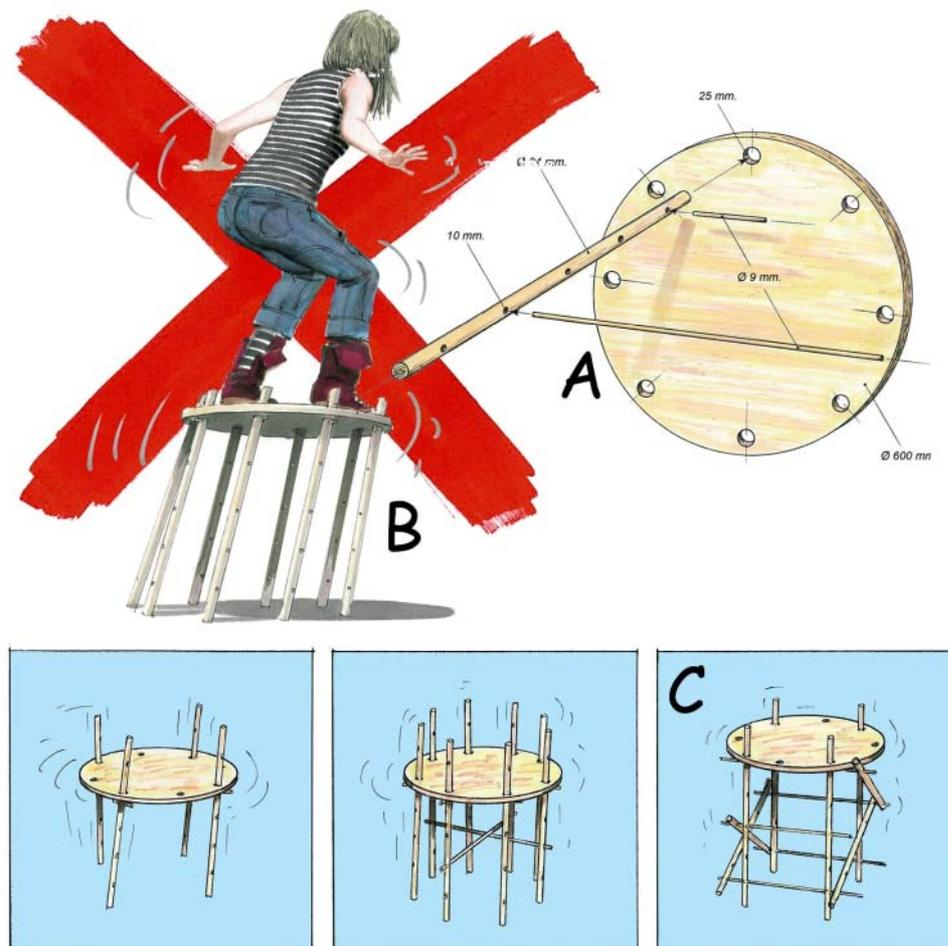
Figure 1: (A) Handstorm<sup>®</sup> Modular Building System parts; (B) Failure of the simple construction of disk and poles and (C) Remedying this by thoughtfully positioning a few connecting sticks.
