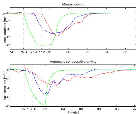
Fig. 11. Comparison of manual and automatic driving during hard braking of the front vehicle
