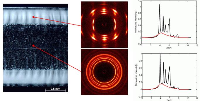
Figure 2 Micrographs at the mid position (left), 2D WAXD patterns (mid) and normalized, integrated intensity curves (right).
