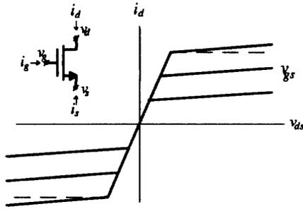
Fig. 1.  $i_d-v_{ds}$  Characteristic of NMOS PL model.
