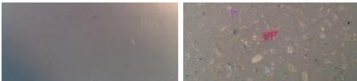
Figure 1: Two samples of homogeneous (left) and heterogeneous (PET contamination, right) PP from sorted household waste.
