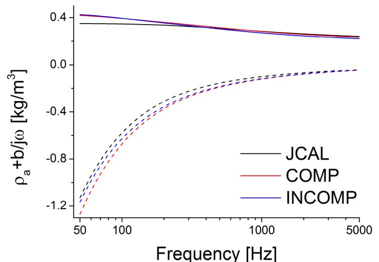
Figure 3. The coupling masses obtained from the JCAL model, the compressible flow model and the incompressible flow model. The solid curves are the real parts and the dashed curves are the imaginary parts.
