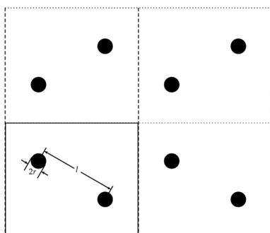
Figure 2. The periodic unit cell (enclosed by the black solid lines) in the simulation. The black solid circles are the motionless solid phase for simplicity. A macro-pressure drop is applied in the horizontal direction.  $l = 884 \mu\text{m}$  and  $r = 161 \mu\text{m}$
