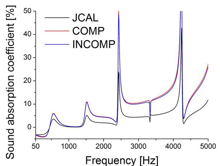
Figure 4. The normal sound absorption coefficient in simulations of a impedance tube by Biot's theory with the coupling masses shown in figure 3.
