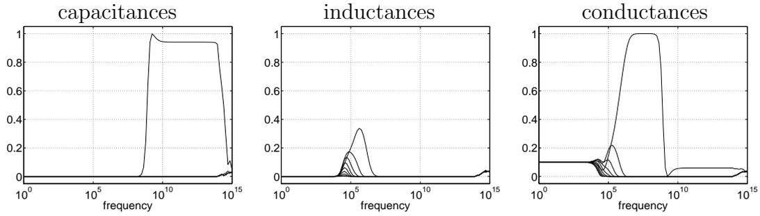
Figure 3: Sensitivities from nonintrusive method ( $N_{\text{cell}} = 10$ ).
