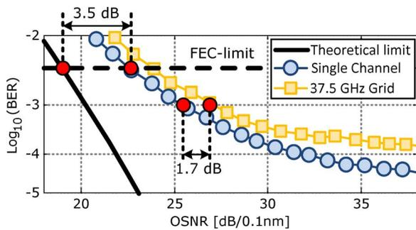
Fig. 2. Measured back-to-back BER curves for 224-Gb/s POLMUX-16QAM.
