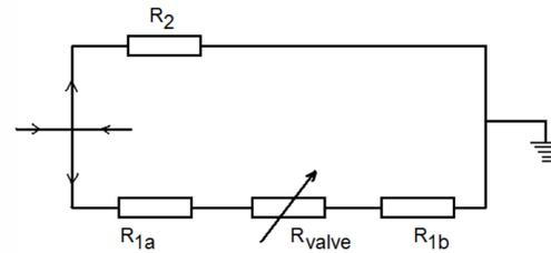
Figure 5: Electrical scheme representing the outflow channels. Ideal values for hydraulic impedances are set by tuning channel dimensions.
