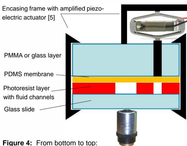
Figure 4: From bottom to top: The objective focuses on the cross-slot, which is created in the photoresist layer with UV lithography. Channel is sealed by the PDMS that also functions as valve membrane.
