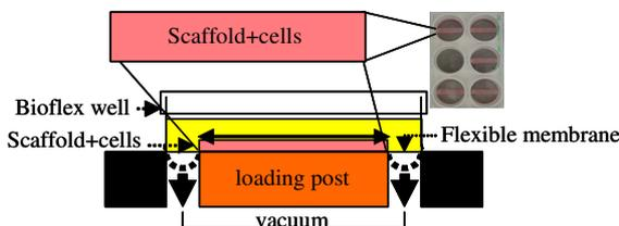
Figure A FlexCell straining device. By applying vacuum, engineered tissues are uniaxially stretched over a loading post.
