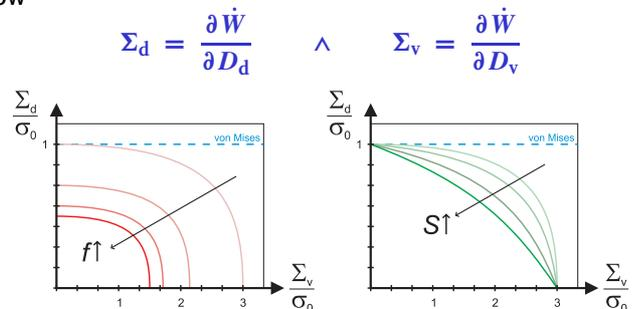
Figure 4 Schematic representation of the non-isochoric yield surface; influence of void size (left) and shape (right).
