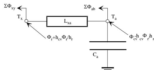
Figure 1 The room model as a thermal network
