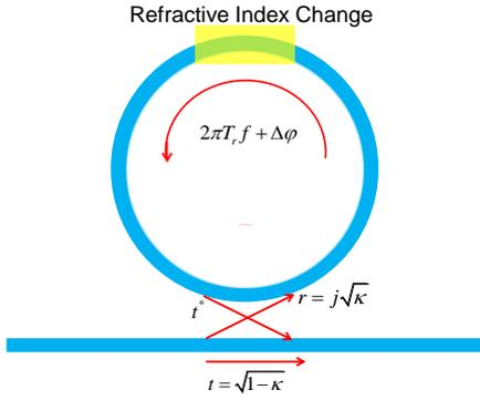
Fig. 1. Principal scheme of the loss-less single MRRs
