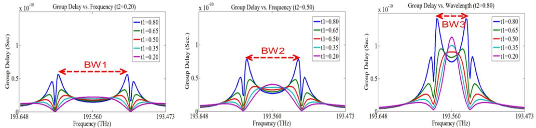
Fig. 7. The group delay response of lattice double chain
