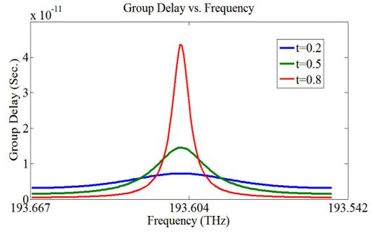
Fig. 2. The group delay response for single MRRs
