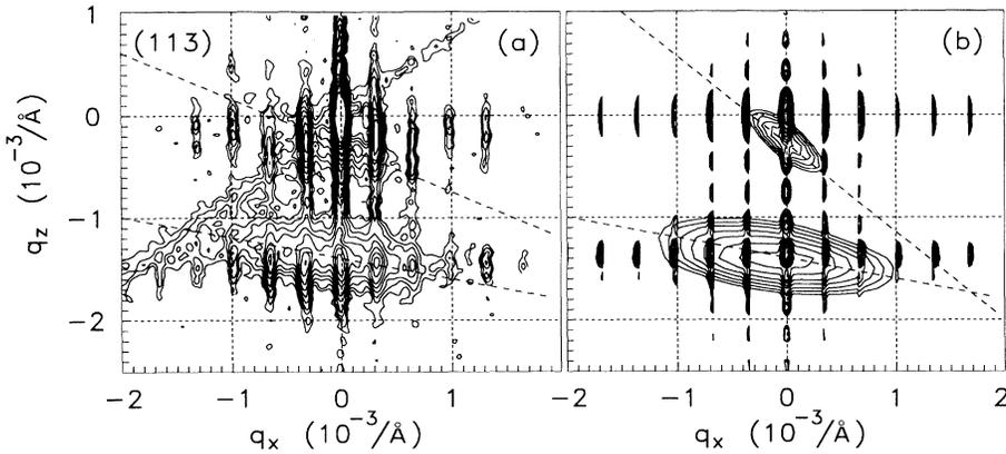
FIG. 7. Measured (113) RSM (low angle of incidence) showing diffuse scattering, which originates both in the GaAs substrate and the MQW structure (a). Simulation (b) using the same set of parameters as determined from the diffuse scattering of the etched MQW. The dashed lines indicate the orientation of the principal axis of the broad diffuse scattering peaks.
