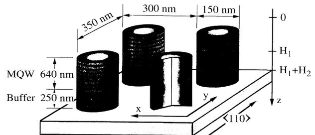
FIG. 1. Schematic diagram of the periodic GaAs/AlAs dot array.
