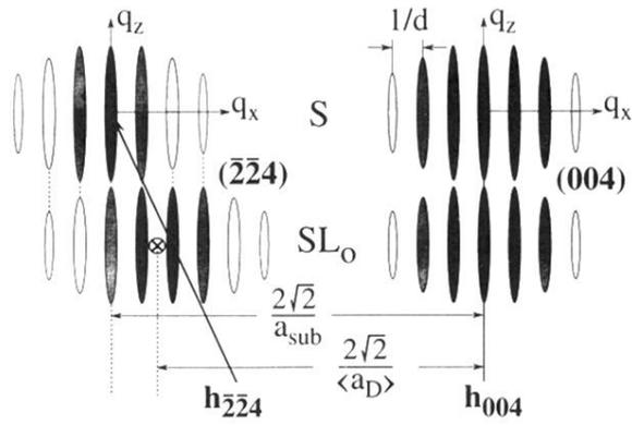
FIG. 5. Schematic sketch of the intensity distribution in the reciprocal plane close to (004) and  $(\bar{2}\bar{2}4)$  reciprocal lattice points,  $\otimes$  denotes the position of the reciprocal lattice point  $(-h_x \varepsilon_{xx}, -h_z \varepsilon_{zz})$  of the dots, i.e., the maximum of the intensity envelope.
