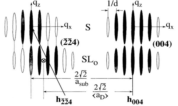
FIG. 5. Schematic sketch of the intensity distribution in the reciprocal plane close to (004) and  $(\bar{2}\bar{2}4)$  reciprocal lattice points,  $\otimes$  denotes the position of the reciprocal lattice point  $(-h_x \varepsilon_{xx}, -h_z \varepsilon_{zz})$  of the dots, i.e., the maximum of the intensity envelope.
