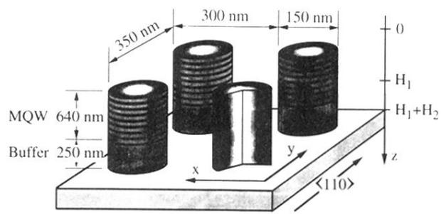
FIG. 1. Schematic diagram of the periodic GaAs/AlAs dot array.
