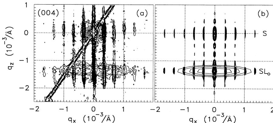
FIG. 3. Measured (a) and calculated (b) reciprocal space maps of the dot array close to the (004) substrate reciprocal lattice point. The intensity scale is logarithmic, the step between two isointensity contours is  $\Delta \log_{10}(I) = 0.2$ . In part (b), "S" and "SL<sub>0</sub>" denote the diffracted intensities originating from the substrate and MQW parts, respectively.
